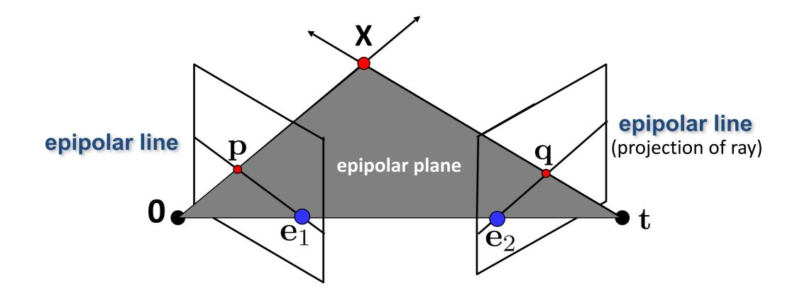
• In camera 1 pinhole frame, 3D point **X** is given by  $\mathbf{X}_1 = \lambda_1 \mathbf{p}$
