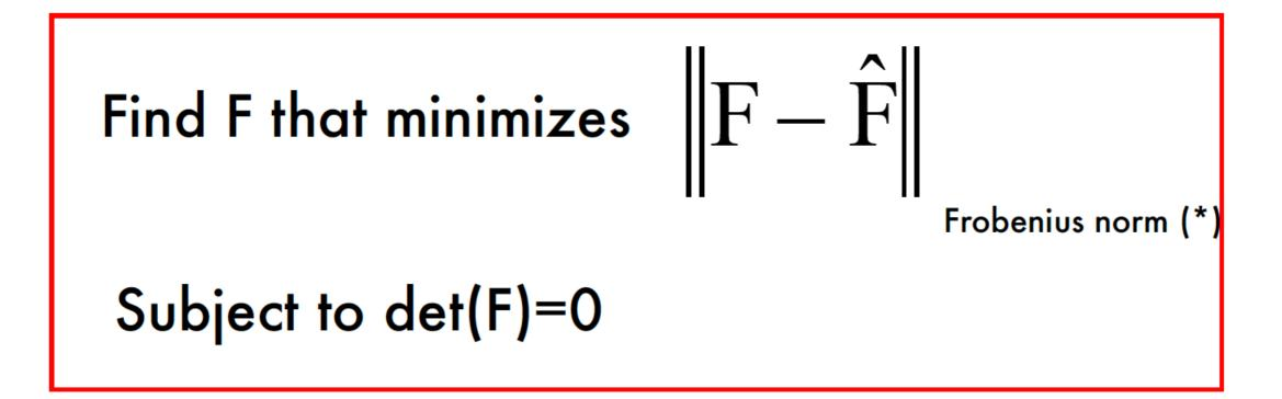
$$F = U \begin{bmatrix} s_1 & 0 & 0 \\ 0 & s_2 & 0 \\ 0 & 0 & 0 \end{bmatrix} V^T \qquad \text{Where:} \\ U \begin{bmatrix} s_1 & 0 & 0 \\ 0 & s_2 & 0 \\ 0 & 0 & s_3 \end{bmatrix} V^T = SVD(\hat{F})$$
